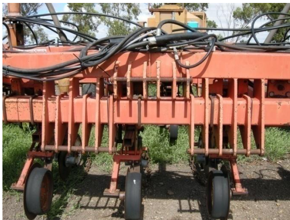
Two 3 point hitches that have been configured for offsetting to suit different row widths
