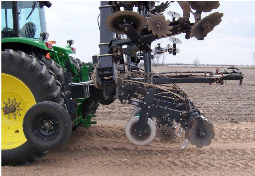
Yetter 8 row strip-till unit with disc opener, trash clearing wheels, fertiliser shank and closing discs.
