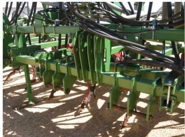
Two 3 point hitches that have been configured for offsetting to suit different row widths
