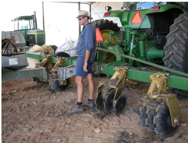
David Brownhill with the machine he uses to rectify CTF tramlines which have been deepened through repeated use.
