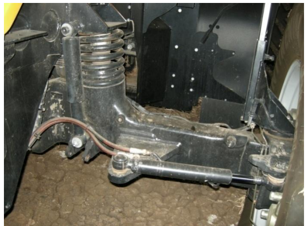
Cast axle extension by Towoomba Engineering
