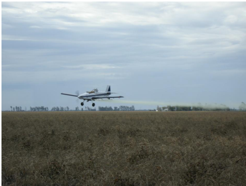
Spray plane applying a UV tracer dye as part of a demonstration to evaluate spray quality.
