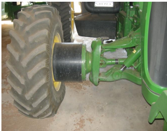
‘Cotton reel’ type axle extension
