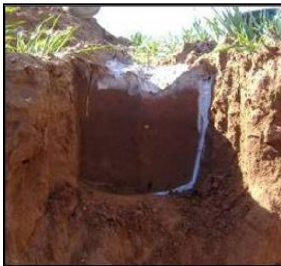
Photo 8 (left). Latex paint on untracked area. Photo 9 (right). Latex paint on tracked area, after one pass of a field sprayer. Source: R. Ruwoldt
