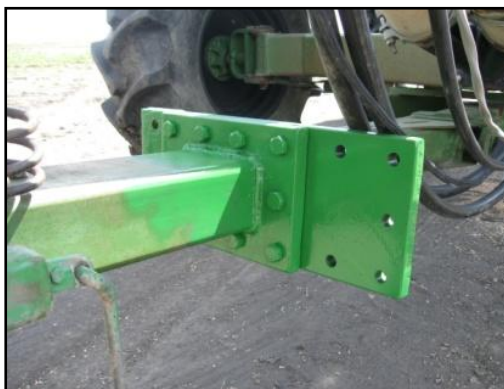
Photo 20 (left). 7.5-inch offset drill hitch. Source: S. Larocque. Photo 21 (right). 6-inch offset air tank hitch. Source: S. Larocque
