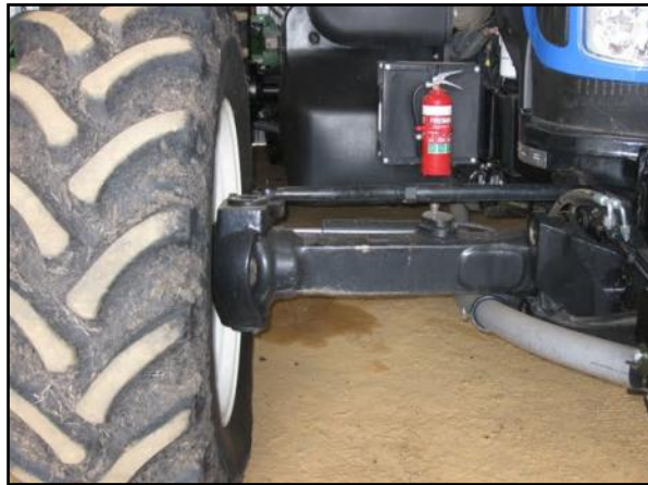
Photo 17. Custom axle extension by C & C Machining, Brisbane. Source: S. Larocque
