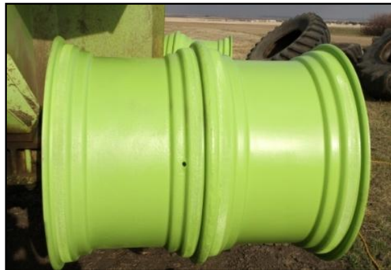
Photo 18 (left). Retrofitted 4WD on singles. Source: S. Larocque. Photo 19 (right). Welded rims. Source: S. Larocque
