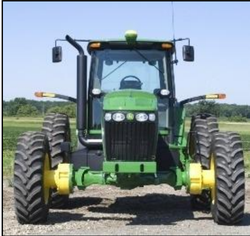
Photo 15 (left). JD 7030 with cotton reels. Source: S. Larocque. Photo 16 (right). John Deere cotton reel kit. Source: John Deere
