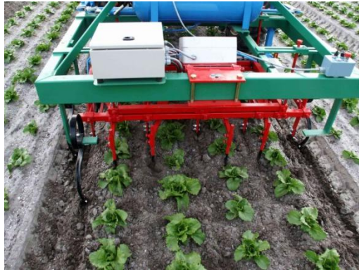
Fig 5.2 Sarl Radis camera guided intra-row weeder.
