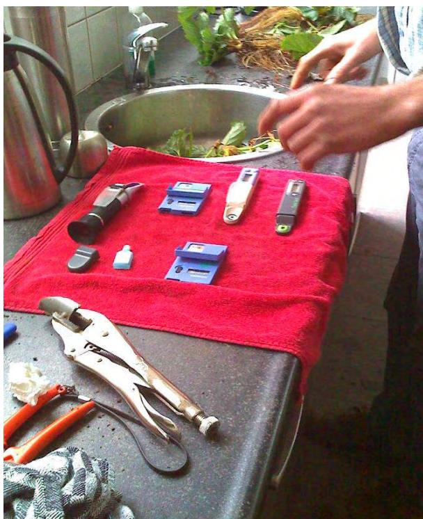
20 Using plant sap tools to monitor plant health.
