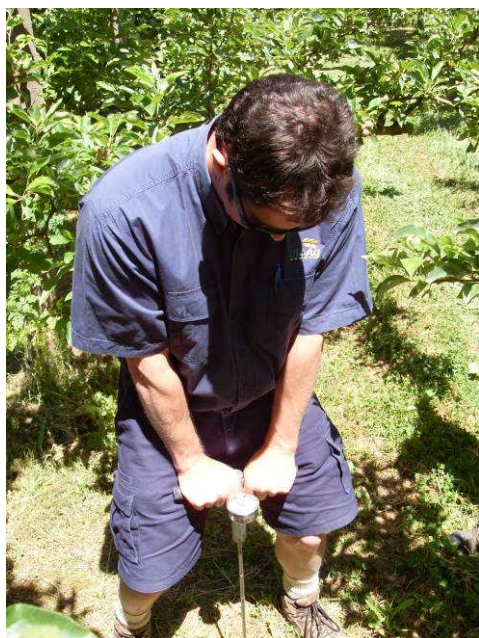
22 Steve Haswell tests for soil compaction using hand held penetrometer
