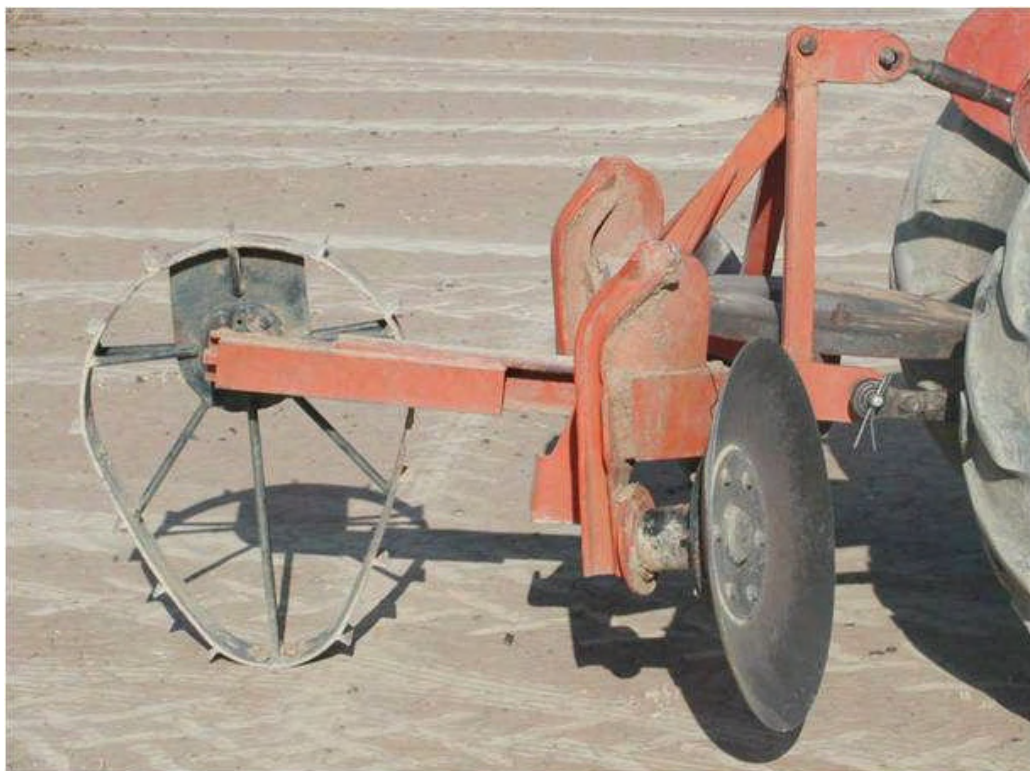
#58 Implement used for scalloping scalded flats in the Karoo Region, showing "egg wheel" for regular pitting effect. Photo c/o Mr. Charl du Plessis, Western Cape Dept of Agriculture.
