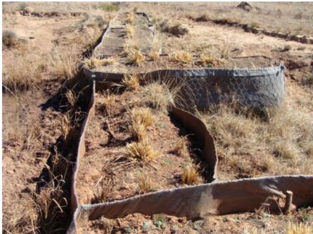
#46 “Earth Basket” trials, by the Free State Department of Agriculture, near Ladybrand, Free State, South Africa. Note eddying out of top section.
