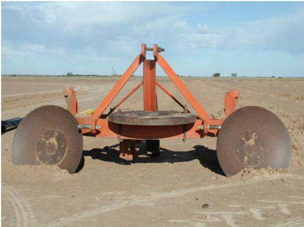
#57 Implement used for scalloping scalded flats in the Karoo Region. Photo c/o Mr. Charl du Plessis, Western Cape Dept of Agriculture, Elsenburg, Western Cape, South Africa.
