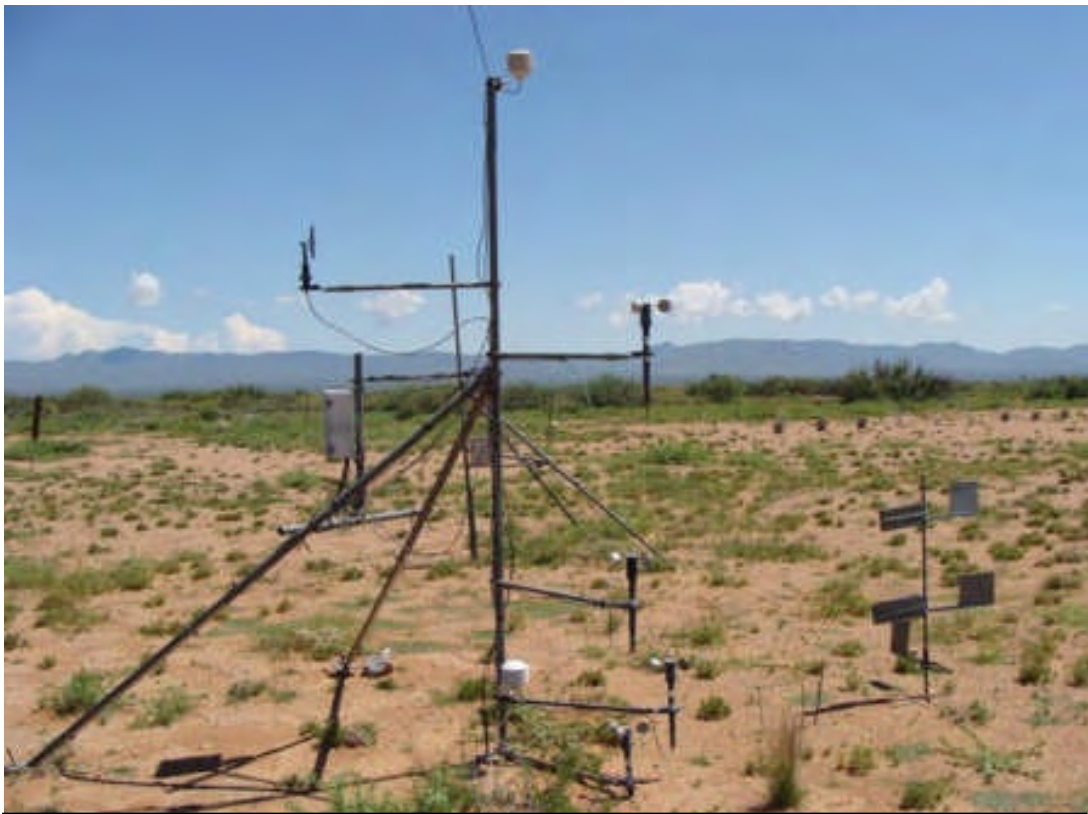
#24 The USDA ARS Jornada Experimental Range. An example of the sophisticated measuring stations around the Range. This set is for measuring erosion caused by wind and the variation of wind effect at different heights.
