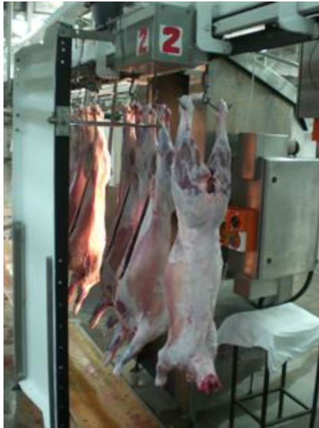
Figure 3 VIAscan VIA system in Lorneville NZ. Note closeness of carcass to camera
