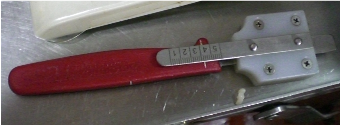
Figure 10 Fat probe used in many Australian and New Zealand abattoirs
