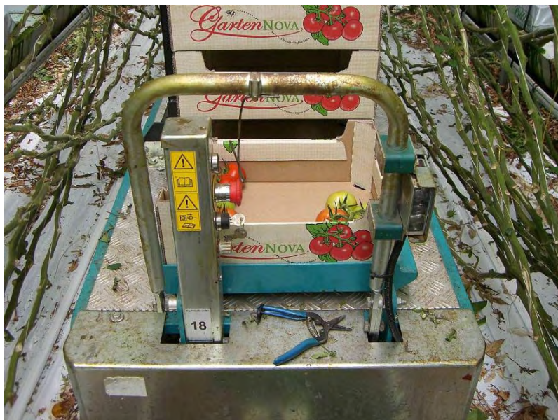
Picture 12. Electronic eye on picking trolley. The Netherlands.
