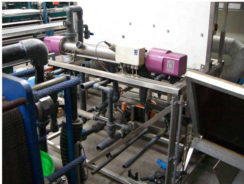
Picture 9. U.V. light sterilising unit. The Netherlands.
