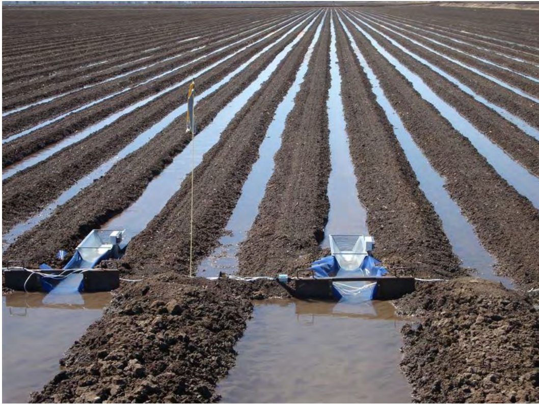
Figure 1: Water-Trac furrow water measuring devices in a planted cotton field.
