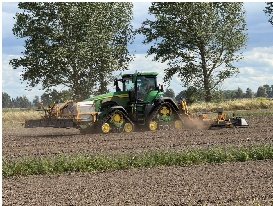
Figure 15 The G's Fresh final pass cultivator has several functions. It applies JS extract before the tines to be stirred into the soil, it lays liquid fertiliser below where the lettuce will be and then sprays a pre-emergent herbicide over the soil pre-planting. (Source: Author)
