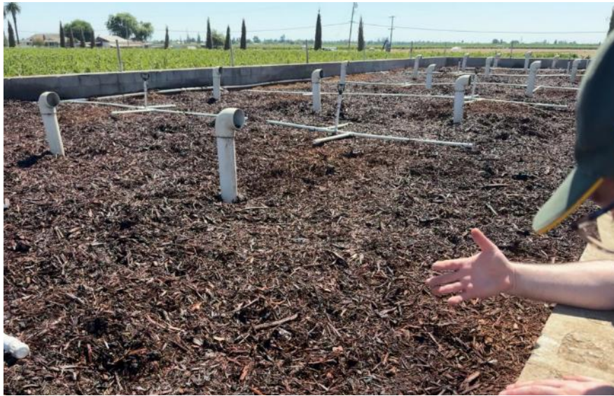
Figure 11 A large scale vermicomposting plant in California. This unusual plant's main role was to filter washings from the vineyard. The outcome was a significant reduction in soluble solids and nutrients. They were captured in the wood chip substrate and cons (Source:Author)
