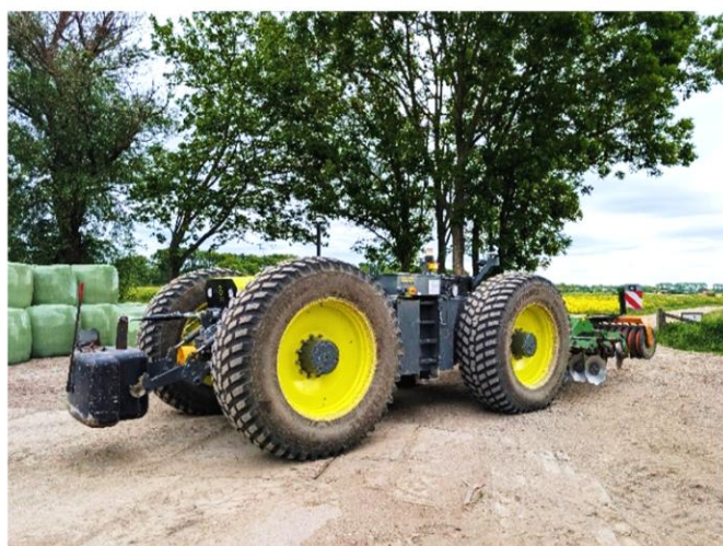
Figure 10: EOX autonomous electric tractor, Netherlands
