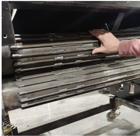
Figure 5.5 Close up of Formation Ag decortication equipment to break apart the shiv and fibre
