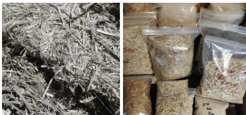
Figure 4.5 'Over-retted' (very dark) hemp straw at Harrison Spinks, Yorkshire and samples of processed fibre and shiv at Formation Ag, Colorado, showing the impact retting time has on colour and quality.
