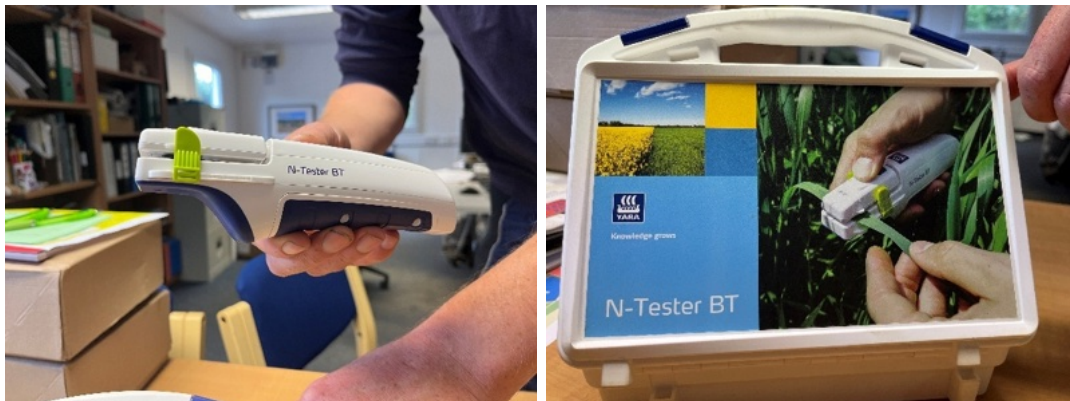
Figures 54 & 55: (From L to R) James Alexander, UK, holding N-tester meter from Yara used to measure nitrogen in cereal crops; box of device (Author, 2024).
