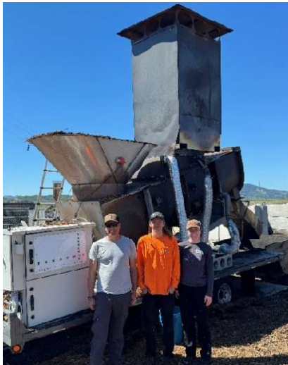
Figure 5. Takachar's trailer-mounted pyrolysis unit (Source: Author)
