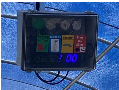
Figure 19 Traffic light timer tells employees when to move to the next stage of the wash process. Source: author’s own
