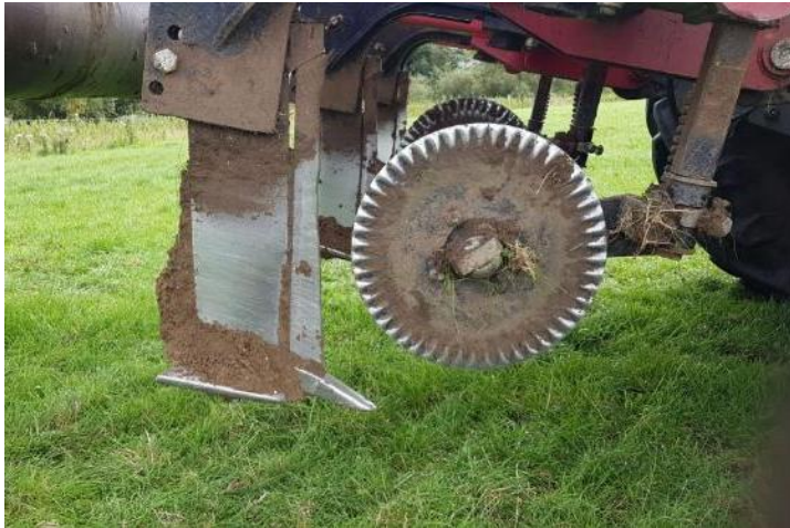
Above: A sward lifter can be used to alleviate compaction at depths of up to 450mm.
