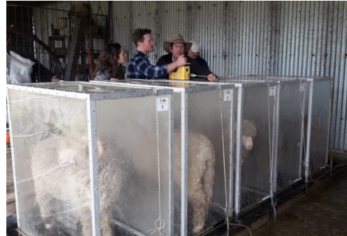
Figure 39: At Instituto nacional de Investigación Agropecuaria Unidad Experimental La Magnolia research facility. Figure 40; reading the gas measurements of the chambers in which sheep were briefly contained (source: author)
