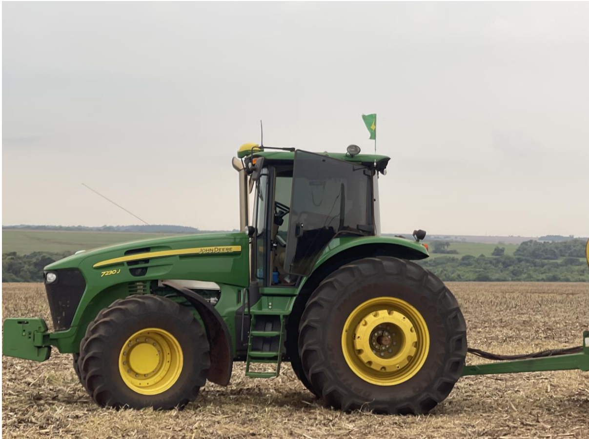
Figure 6: John Deere tractor drilling soya utilising satellite technology for yield mapping, variable rate applications and autosteer in Maracaju, Brazil. Photo: author's own.
