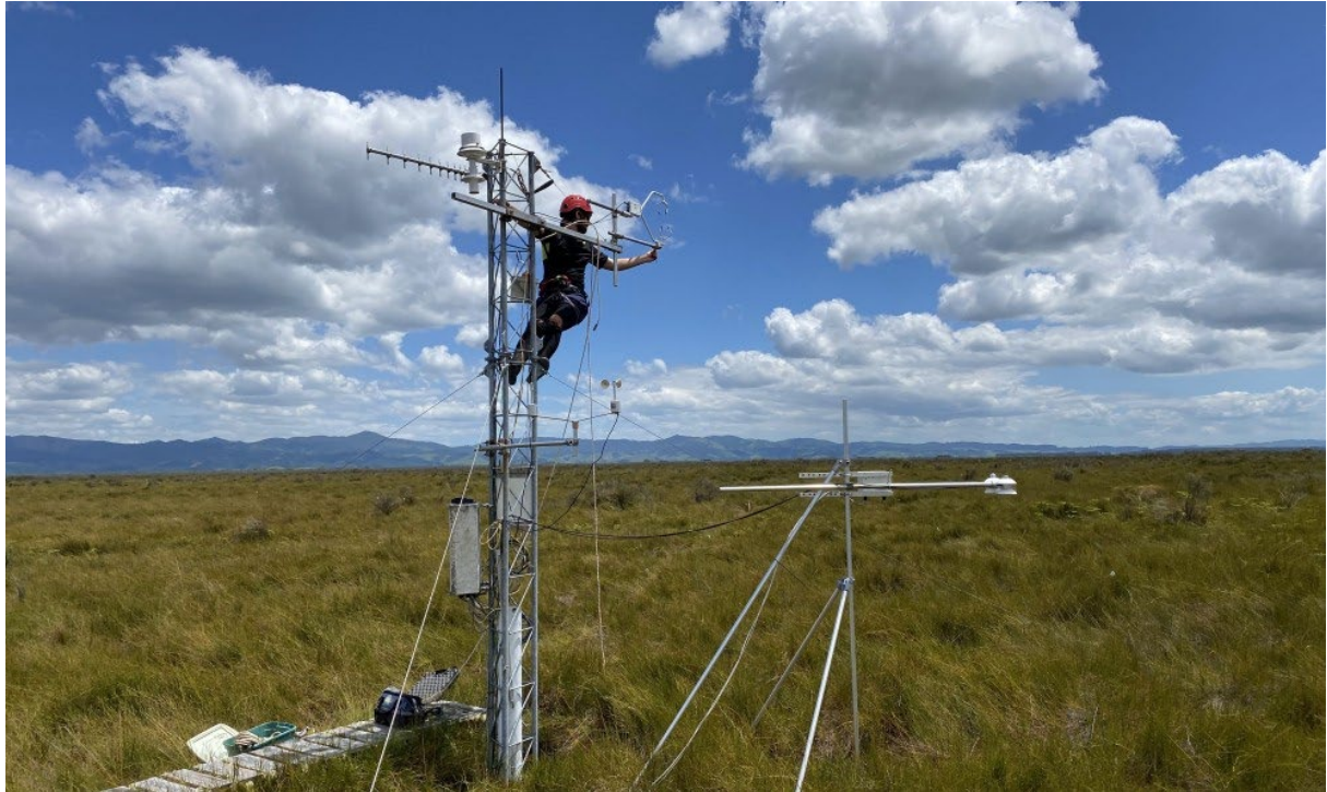
Photo 2: Dr. Dave Campbell at the flux tower in Kopuatai Peat Dome, the largest raised bog in NZ. Instruments at this tower measure carbon dioxide exchange between the peatland and the atmosphere, providing data on carbon sequestration (photo credit: G. Glover-Clark)
