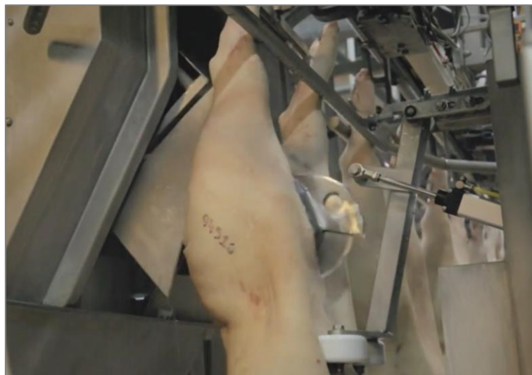
Figure 4 - Robots process pig carcasses (Source: Danish Crown virtual tour)
