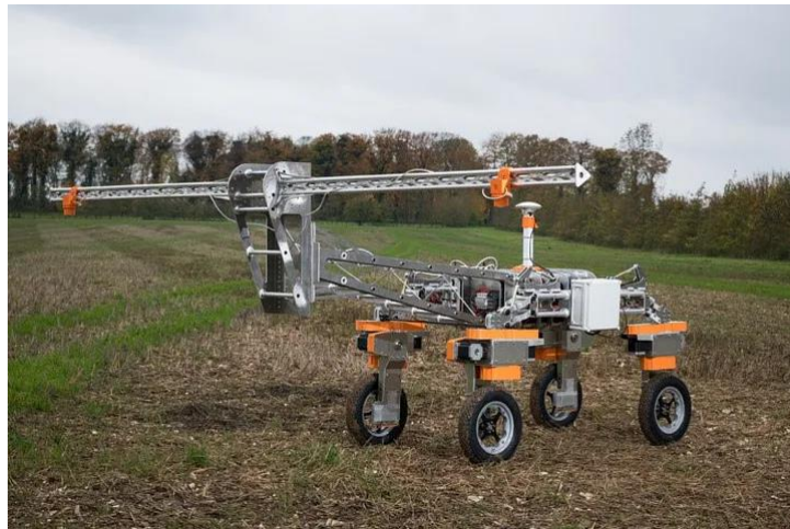
Figure A.10 – Small Robot Company weed mapping robot (Source: The Engineer )
