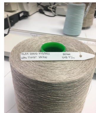
Figure 4: The finest Safilin yarn 50 Tex 245 T/m
