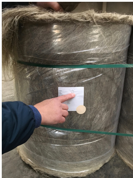
Figure 12: A 100kg bale of long line flax showing the traceability (origins) and exact weight in Belgium at Albert Brille's scutching mill
