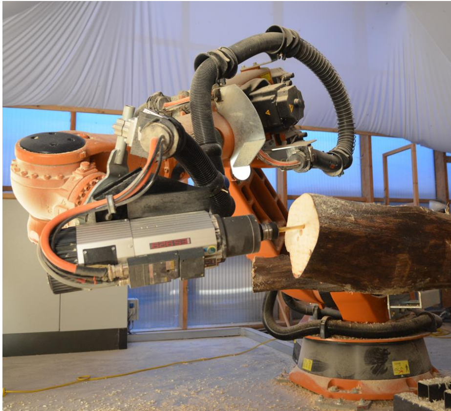
Figure 95: A robotic milling machine adapts a forked piece of timber to the necessary dimensions and forms joints. Photo: Architectural Association.
