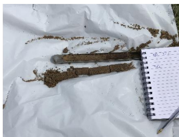
Figure 7: The sandy soils of Florence showing non-tillage (top core) and tillage (bottom core) treatments, Florence, SC, March 2019 (Image: Author)
