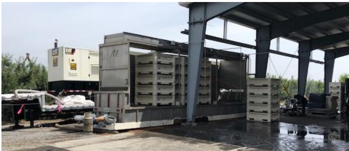
Figure 7: Mobile hydrocooler at loading bay, Washington State, USA (Author, 2019)
