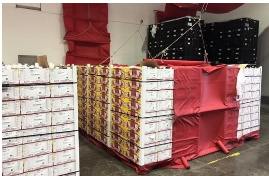
Figure 13: Tunnel-style forced air cooling of stone fruit, HMC, California, USA (Author, 2019)
