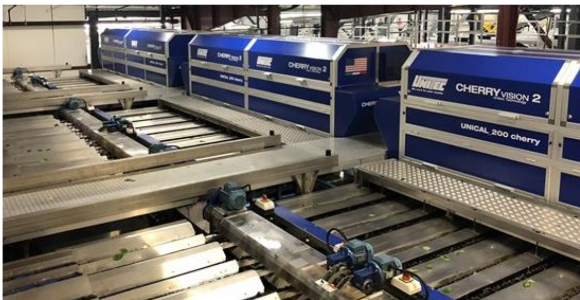
Figure 11: Unitec Cherry Vision 2.0 optical grader, Orchard View, Oregon, USA (Author, 2019)
