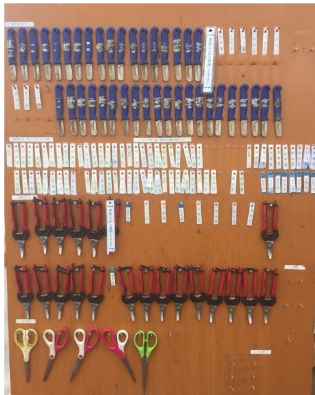
Figure 6: Asai nurseries shadow board for all harvest tools Source: Author (2018)
