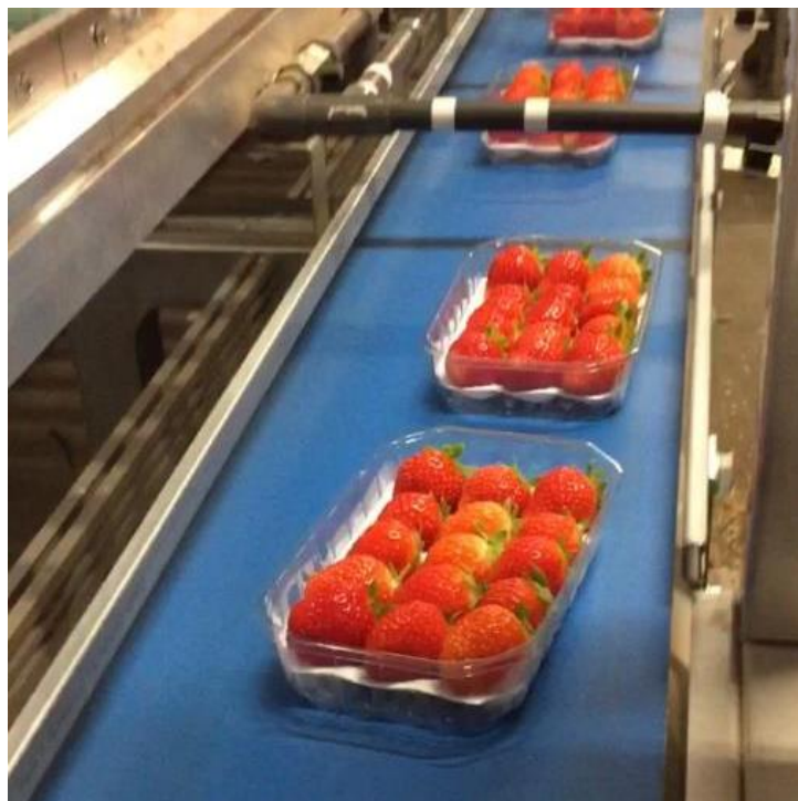
Figure 8: Strawberries being packed at Brookberry for the Japanese market. Compressed air being blown on the strawberries to remove dead leaves Source: Author (2018)
